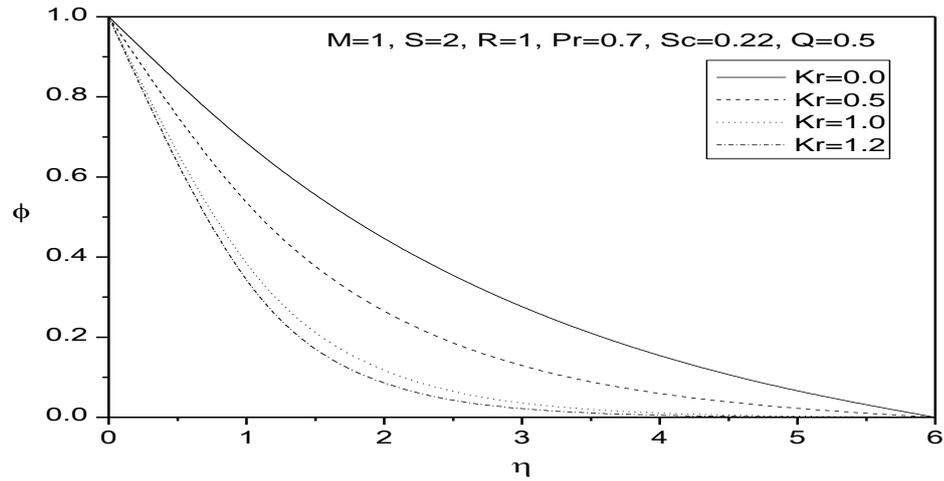
Fig. 11. Concentration profiles for different values of  $kr$
