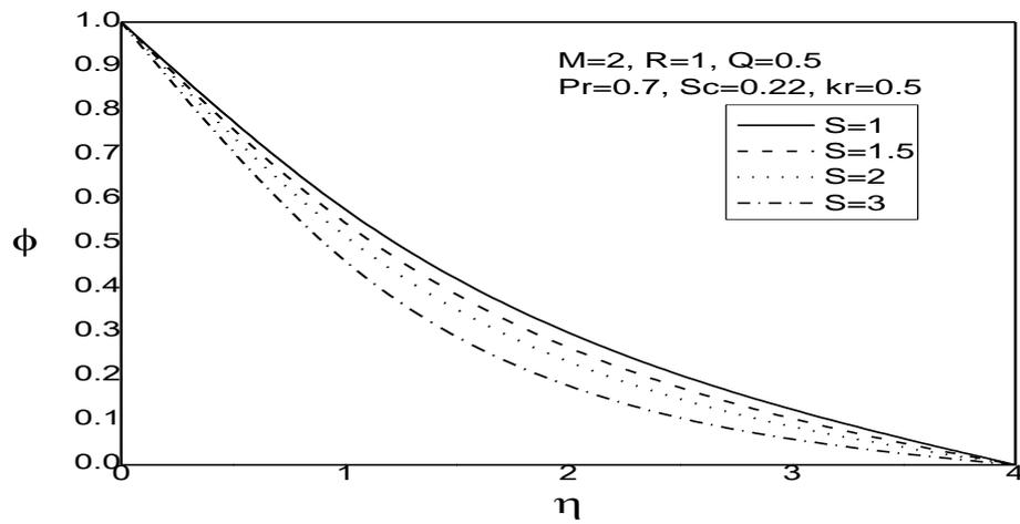
Fig. 9. Concentration profiles for different values of  $S$
